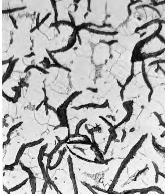
Figure :4.2 Gray iron: the dark graphite flakes are embedded in an -ferrite matrix
